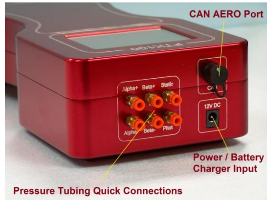
Figure 2: FTK100 Top Panel Features
